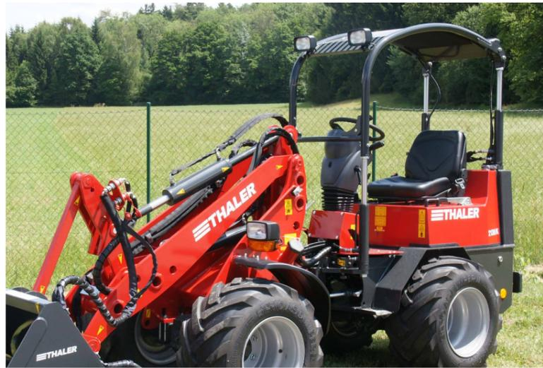
Hydraulically in height adjustable 4-post-Rops-Fops protection cage.
