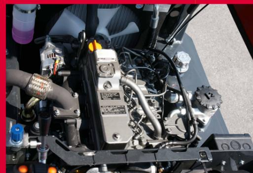
Smooth running Yanmar engines, accessible by 3 sides thanks to the operator's platform tiltable to the rear by 90°.
