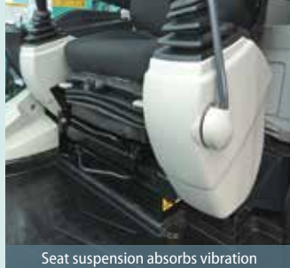
Seat suspension absorbs vibration
