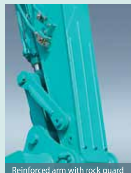
Reinforced arm with rock guard
