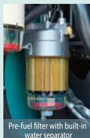
Fuel filter with built-in water separator
