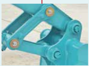
Bucket Cast-iron idler link provide greater strength.
