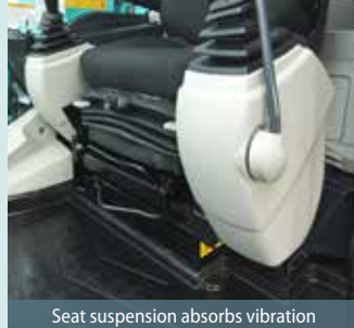
Seat suspension absorbs vibration
