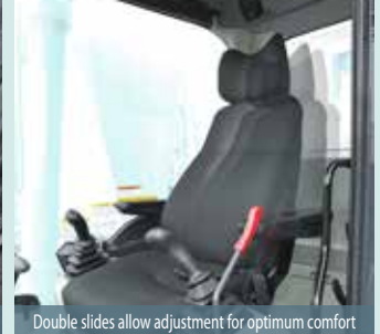
Double slides allow adjustment for optimum comfort
